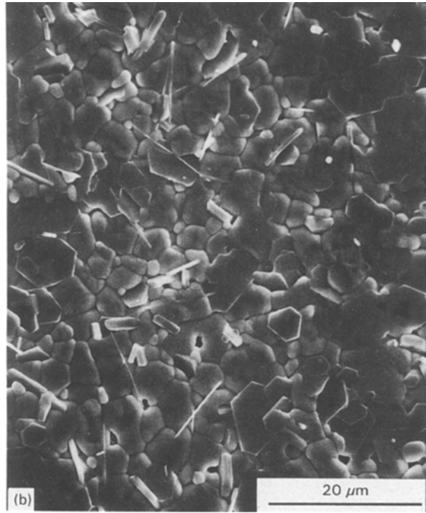
Figure 1 SEM micrographs of PTC26/74 ceramics: (a) A1, (b) B1, (c) C1.
